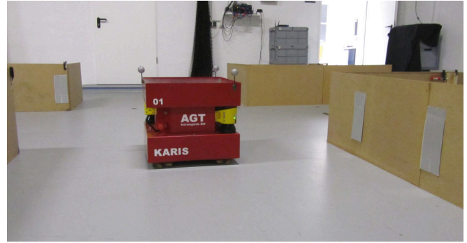
Fig. 1. The KARIS robot in the experimental environment. The two laser scanners on opposite corners of the robot provide a 360° field of view. The three stripes of reflective tape on the walls can be detected in the laser scans and are part of the robust landmark set selected by our approach.
