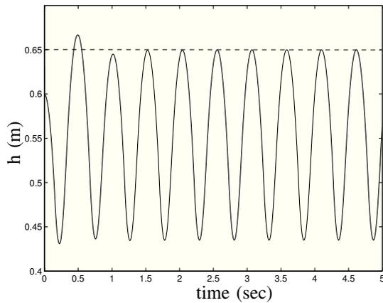
Fig. 2. Center of mass height above the ground for the four-link hopper
