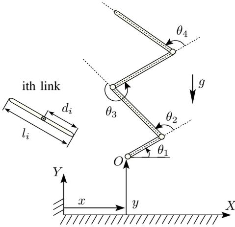
Fig. 1. Four-link hopping robot
