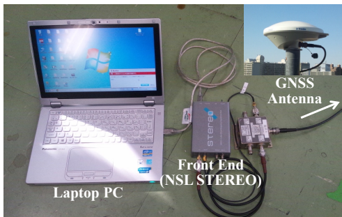
Figure 4. Set-up of software GNSS receiver.
