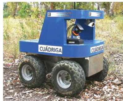
Fig. 4. Quadriga mobile robot with onboard 3D rangefinder.
