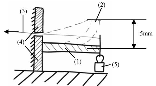
Figure 11. Test setup with tested structure (1) and the actuated tip (2), Bowden wire (3), a base (4) and the weight (5).
