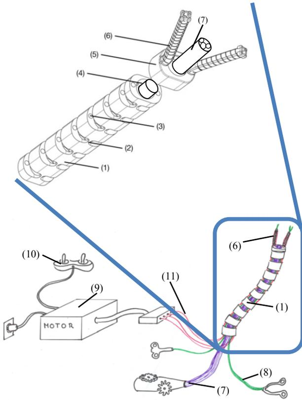
Figure 1. Concept of the Multi Arm Snake-Like Robot System with a frame (1), 1D flexure hinges (2), two instrument channels (3), one channel for a standard flexible endoscope (4), an adapter (5), manipulator arms in helical shape (6), a flexible endoscope (7), flexible instruments (8), motors (9), a joystick (10) and the actuation Bowden wires (11).
