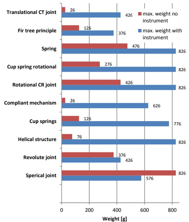
Figure 14. Results of the experiment: maximum weight load compared with all structures. Red is without instrument and blue with inserted flexible endoscopic instrument.
