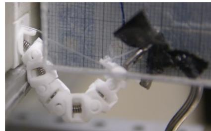
Figure 15. Broken kinematic: revolute joints with inserted instrument, broken at the shaft of the structure with a loaded weight of 476 g.
