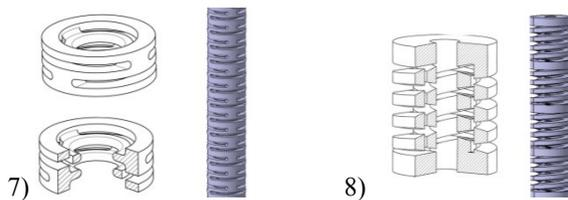
Figure 7. Circular leaf springs (7) are two plane cup springs connected with 90° shift. Two springs with shifted pitch and limited end stop are shown in (8).
