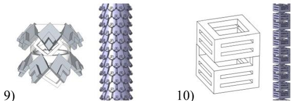
Figure 8. Fir tree principle (9) is a structure with cup springs inside and end stops at the outside and the CT-joint (10) based on translational flexure hinges.
