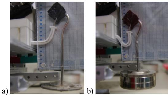
Figure 13. Spring cups during the experiment. a) with the load of the base and b) with base and a weight of 250g.
