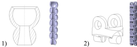
Figure 4. Rigid bodies: spherical- (1) and revolute joints (2), both designed with an air gap of 0.3mm between the moving parts. The structures should be manufactured monolithically (one piece).
