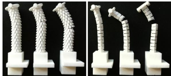
Figure 16. Specimen after the experiment; three of each type: a) fir tree principle and b) CT-Joint structure.
