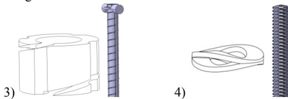
Figure 5. Flexure hinges: helical structure (3) is a cylinder with a continuous helical flute, to weaken the structure and to create the necessary flexibility. The cup springs (4) are bended cup springs, the flexibility is created by the change of flexible (loose) parts and stiff (connected) parts of the structure.
