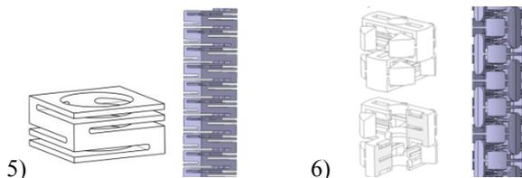
Figure 6. Compliant mechanisms (5) realized by a weakened bar and CR-joints (6) based on rotational flexure joints.
