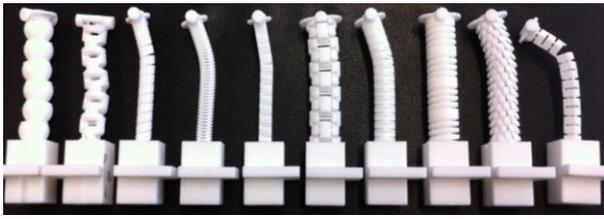
Figure 17. All specimen after the experiments: from left to right: spherical joints (1), revolute joints (2), helical (3), cup spring (4), compliant mechanism (5), CR-joint (6), rotational cup spring (7), spring (8), fir tree (9) and CT-Joint (10).
