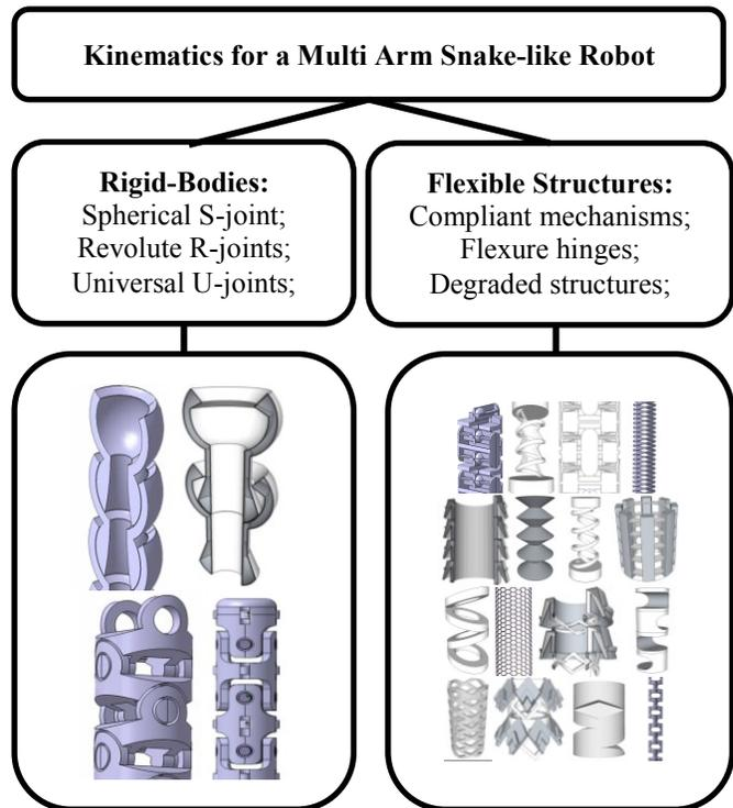
Figure 3. Overview of design principles and realized designs (lower pictures) to build a Multi Arm Snake-Like Robot: left: real joints (manufactured in one part: monolithic), not assembled or glued and right: different shapes of kinematics based on flexure hinges. Structures on the right are flexible joints based on the flexibility of the used material.
