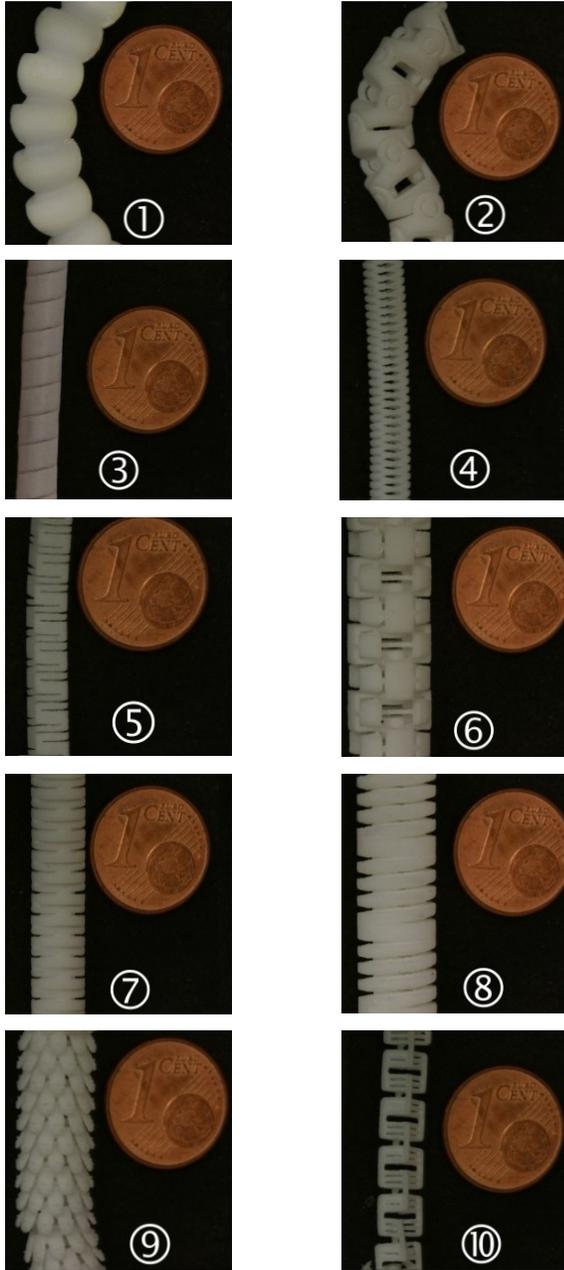
Figure 10. Realized structures: spherical joints (1), revolute joints (2), helical structure (3), cup springs (4), compliant mechanisms (5), revolute CR-joints (6), circular leaf spring (7), spring (8), fir tree principle (9) and translational CT-joint (10).
