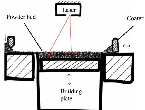
Figure 9. Principle of Selective Laser Sintering (picture source [11]).
