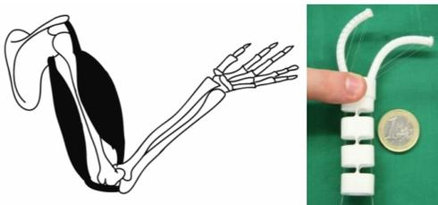
Figure 2. Nature mimicry: the actuation of the system can be compared to the human arm. The cables on the outside (muscles) are actuating the structure inside (bones).
