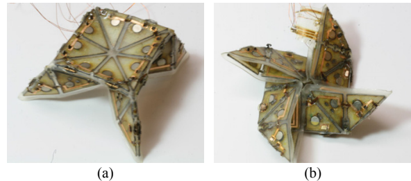
Figure 1. Examples of different shapes a Robogami can transform into (a) a table (b) a pinwheel.
