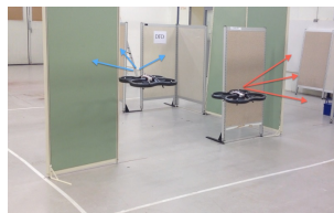
Fig. 1. Motivating example: Two UAVs are cooperatively examining targets in two separated rooms. The task-sequence assignment from UAVs to targets, i.e., each robot's set of targets and the sequence of visiting them, is computed by human-assisted optimization introduced in this paper.
