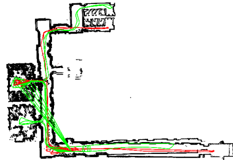
Fig. 7: Experiment at the DIS building of La Sapienza University of Rome. The misalignment observed in the bottom right corner originates from the fact that the robots never meet in that region, thus they are unable to determine constraints between that part of their trajectories. This can be recovered when the two robots meet in that region, or in a post-processing phase.
