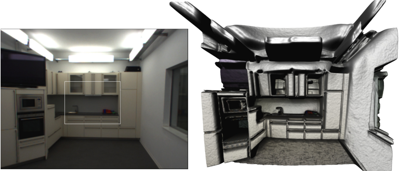
Fig. 5. Visual manifold acquisition. The HDR mesh is the \ln(E) compressed representation of the radiance scene acquired with VGA resolution using the 4mm lens, see also the integrated HDR acquisition pipeline in figure 1). The total acquisition time of this HDR image is 6.672 sec fusing 11 exposures with 16 samples during the temporal fusion per iso-exposure. When fusing only one out of ten (1/10) exposures of the total 651 (available in camera) it takes 34.236 sec to acquired the HDR image. When capturing with less than (1/10) exposures the result presents holes in the high range regions of the images, for instance at laps or in the ceiling, see marked zone in figure 6. This means a 513.11% time performance improvement compared to the 1/10 regular distributed (naive exposure) plan.
