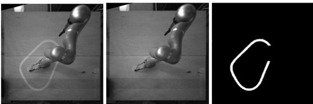
**Figure 9: Computation of current-state mask (right) by differentiation of light (left) and dark (mid) image.**
