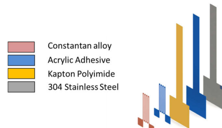
Figure 7. Gage layout on the top structural layer
