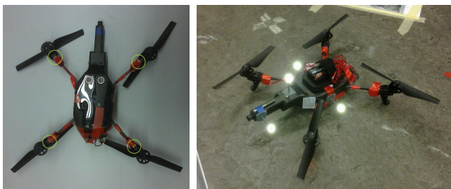
Fig. 6. The ARDrone 2.0 equipped with four ALMs (shown in a) tracked by the DVS, and reflective markers used by the OptiTrack (shown in b).
