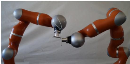
Fig. 5: Experimental configuration in 1 DoF: right-hand side robot is providing a variation of stiffness (softening) at the single point contact along the  $y$  axis of the left-hand side robot.
