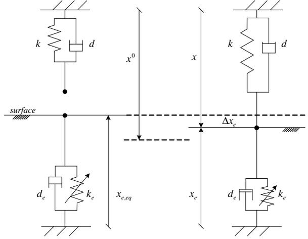
Fig. 3: Unidimensional model of interaction with unknown environment stiffness.
