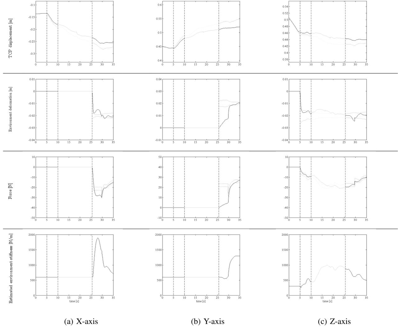
Fig. 8: Assembly task results (translational components). (top) commanded (dotted line) and measured position (solid line) of controlled TCP; (mid-top) desired band of (dotted line) and obtained (solid line) deformation of environment; (mid-bottom) desired band of (dotted line) and obtained (solid line) interaction force; (bottom) estimated environment stiffness.
