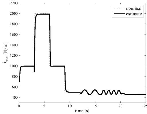
Fig. 4: Stiffness estimation in simulation experiment in 1 DoF, along a vertical axis.
