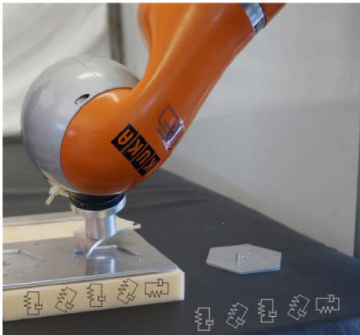
Fig. 1: Compliant KUKA LightWeightRobot inserting shapes (unknown to the controller) on partially unknown substrate. The environment is made by two different material with unknown mechanical properties and unpredictable shear.
