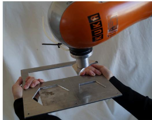
Fig. 7: Compliant KUKA LightWeightRobot inserting shapes (unknown to the controller) while an operator is holding the substrate. The environment preserve passivity to some extents and is naturally time-variant.
