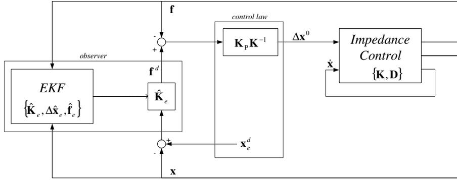
Fig. 2: Deformation-tracking with impedance control: reference trajectory  $\Delta \mathbf{x}^0$  for Cartesian impedance controller id defined by a *control law* using a force-tracking derived from deformation-tracking on the basis of environment estimation by the *observer*.
