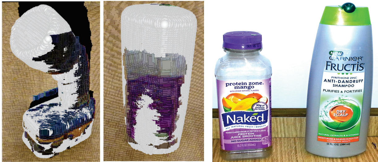
(a) Point clouds with RGB texture from the vision system. On the left is a flashlight along with its aligned point cloud in white. On the right is the point cloud of a juice bottle along with the best model from the vision system's object database, a shampoo bottle, in white. (b) The juice bottle on the left is used as a novel object in this experiment. In Fig. 2 and Fig. 5(a), we show the model of the shampoo bottle aligned with the point cloud data from the juice bottle. Although the objects are relatively different in size and shape, the alignment found by the vision system is sufficient to run the grasp planner on the bottle.
