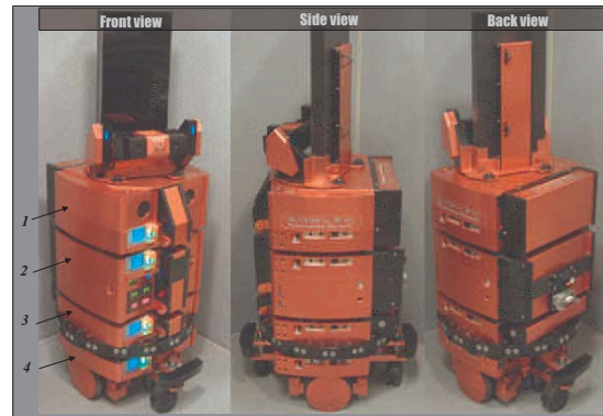
Fig. 11. Robot adopting proposed suspension mechanism. 1, 2, 3, and 4 represent a recognition, an arbiter, a sensor, and a mobile module, respectively.
