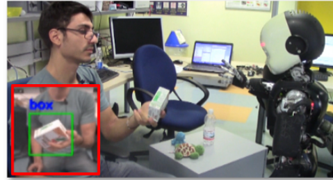
Fig. 1. The Human Robot Interaction setting for the data acquisition. Independent motion detection provides a good estimation for the object position in the image.
