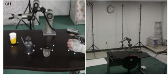
Fig. 5. Illustrations of a robot arm and a motion capture system: (a) Katana robot arm and four objects (i.e., cup, kettle, teabag, and human hand) and (b) Experimental environment containing a robot arm and a motion capture system.
