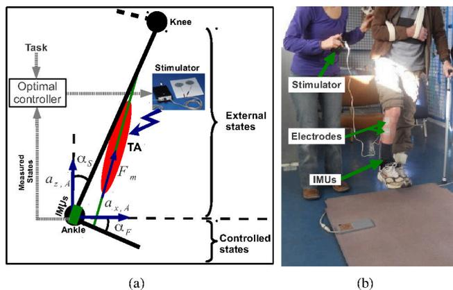
Fig. 1. Experimental setup of the FES-based DFC. (a) Optimal control prototype for DFC and model of ankle joint controlled by electrically stimulated Tibialis Anterior (TA) muscle and influenced by external states ( $\mathbf{x}^{ext}$ ). (b) Hemiplegic subject and equipments used in experiments for inertial data acquisition.
