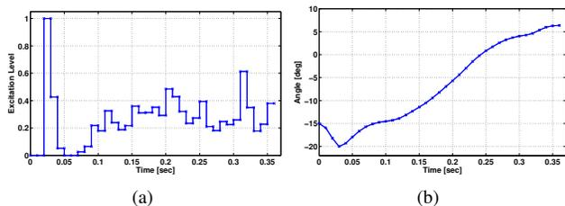
Fig. 6. NMP control results with an adaptive foot orientation constraint, which depends on the position of the ankle (real data); (a) The muscle excitation ( $u_1$ ); (b) The foot orientation angle ( $x_2$ ).
