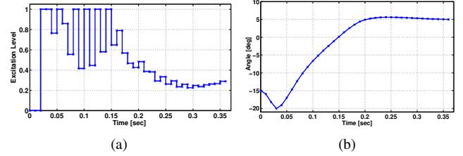
Fig. 4. NMP control results with a fixed constraint of foot orientation. (a) The muscle excitation ( $u_1$ ); (b) The foot orientation angle ( $x_2$ ).
