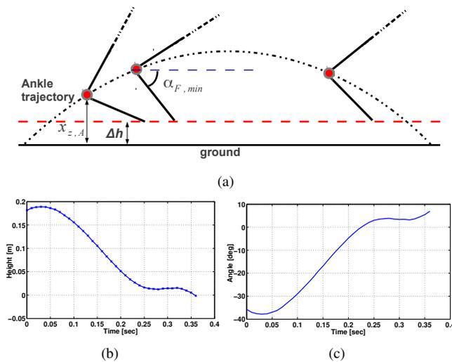
Fig. 5. Model of foot orientation adaptive constraints (a), real data of ankle heights (b) and the calculated adaptive minimal foot orientation  $\alpha_{F,min}$  (c).
