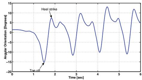
Fig. 2. Absolute shank orientation obtained by integration gyroscopic measurements.
