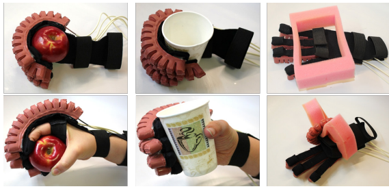
Fig. 11. Using the soft glove to grasp various objects.
