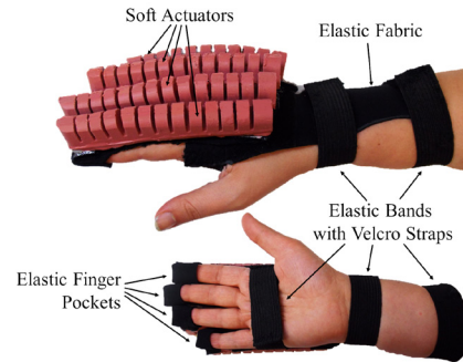
Fig. 10. Top and bottom views of the prototype showing the soft actuators and the open palm glove configuration with the Velcro straps.
