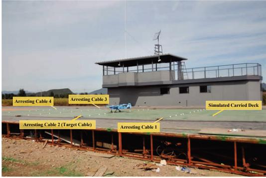
Fig. 11. Simulated Carrier Deck.
