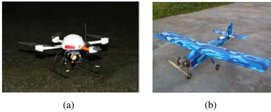
Fig. 2. (a) md4-200 quadrotor platform (b) fixed-wing platform
