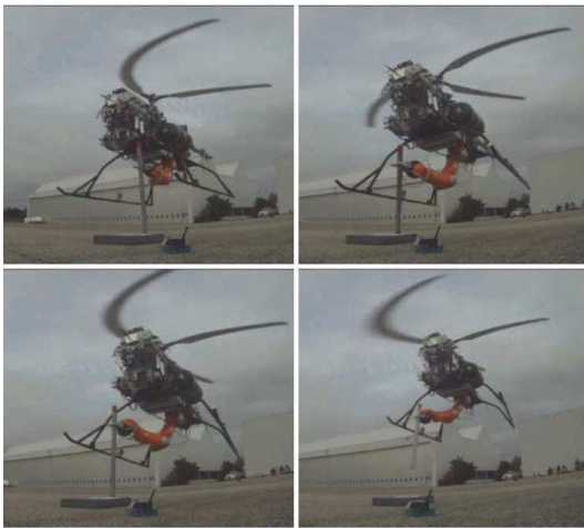
Fig. 13. This sequence shows the robot arm compensating the helicopter movement during the grasping task.
