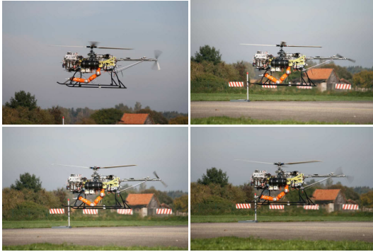
Fig. 12. Snapshots of manipulation task. Helicopter is arriving at the target area, hovering with activated vision system and grasping the pole.
