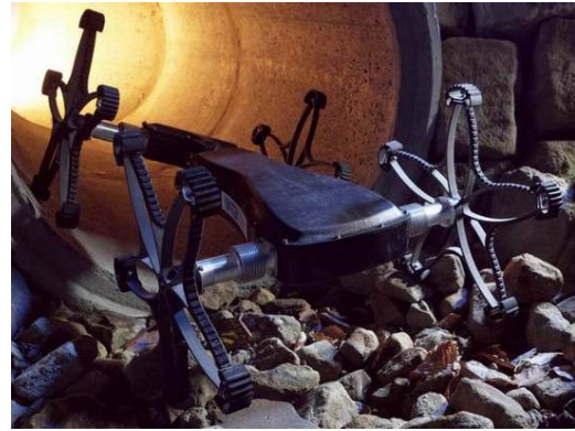
Figure 1. Asguard high mobility rover by DFKI [3]
