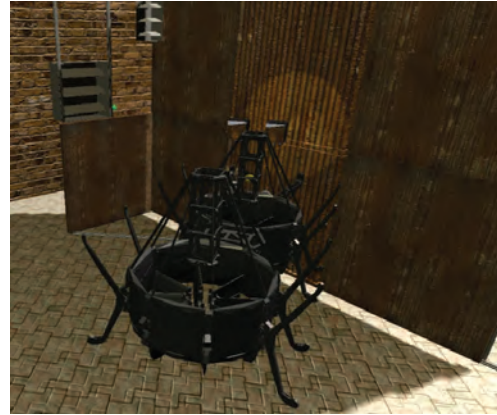
Fig. 1. Typical inspection-by-contact task performed by the “double” ducted fan.
