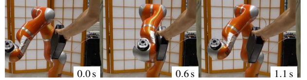
Fig. 9. If the capacitive sensing system measures in single-ended mode, the empty plastic case cannot be detected early enough to avoid a collision. Thus the arm touches the object before it moves back.
