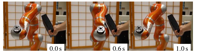
Fig. 10. When using the capacitive sensor in differential mode, even an empty plastic case can be detected early enough to avoid a collision.
