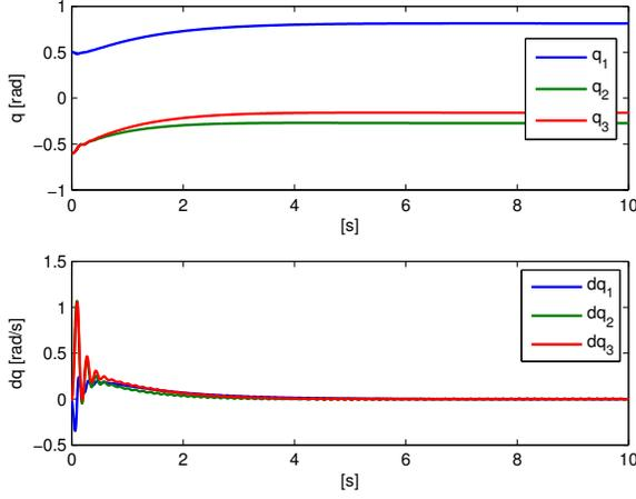
Fig. 3. Case 1: Joint position and velocity of the robot manipulator
