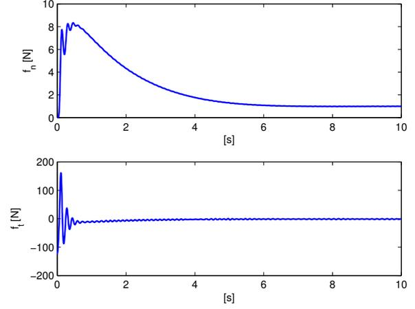
Fig. 5. Case 1: Convergence of normal and tangential forces. Notice that the shape of these forces are, as expected, highly correlated to deformation and angle transient, see Fig. 6.
