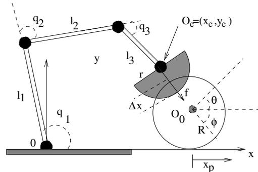
Fig. 2. Circular object manipulation over a rigid surface.
