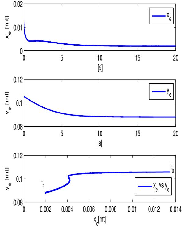
Fig. 8. Case 2: Smooth convergence to the regulation point by the deformable soft fingertip which is interpreted also as the hemispherical fingertip is rolling, with the phase plane  $(x_e, y_e)$  shown in the bottom.
