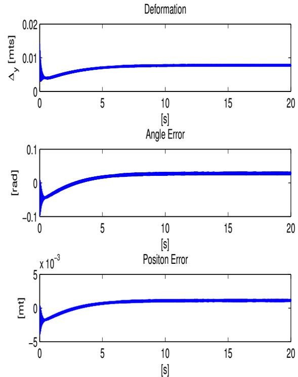
Fig. 10. Case 2: Soft finger-tip penetration along its maximum radial deformation, top, with the convergence of rolling angle, middle, and position error, bottom.
