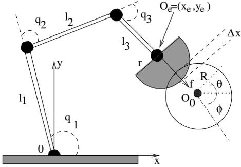
Fig. 1. Kinematic parameters of the circular object pivoting around  $O_0$ , where  $O$  is the origin of the world reference frame,  $O_e = (x_e, y_e)$  is the center position of the base of the deformable soft fingertip of radius  $r$ . Furthermore,  $\mathbf{q} = [q_1, q_2, q_3]^T$  stands for the generalized angular position coordinate,  $R$  is the radius of circular object and  $l_i$  is the length of each link  $i$ .
