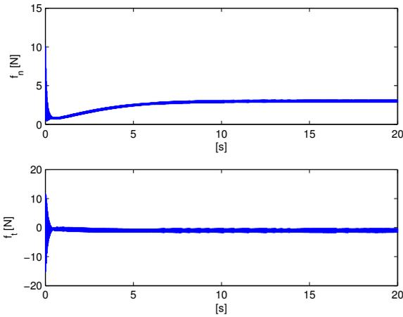
Fig. 9. Case 2: Normal force converges in about 10s while the tangential forces converges in few seconds to prevent slippage of the freely moving dynamic object. For the same reason, it shows a very small high frequency value coming from its corresponding position error along the tangent direction, see bottom of Fig. 10.
