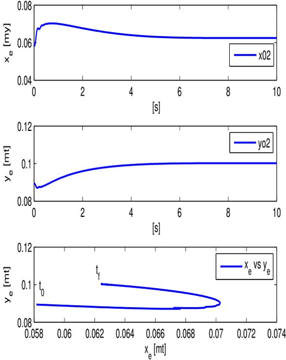
Fig. 4. Case 1: Displacement of rolling angle can be seen through how the center position of the base of the deformable soft finger-tip is moving, with the phase plane  $(x_e, y_e)$  is shown in the bottom.
