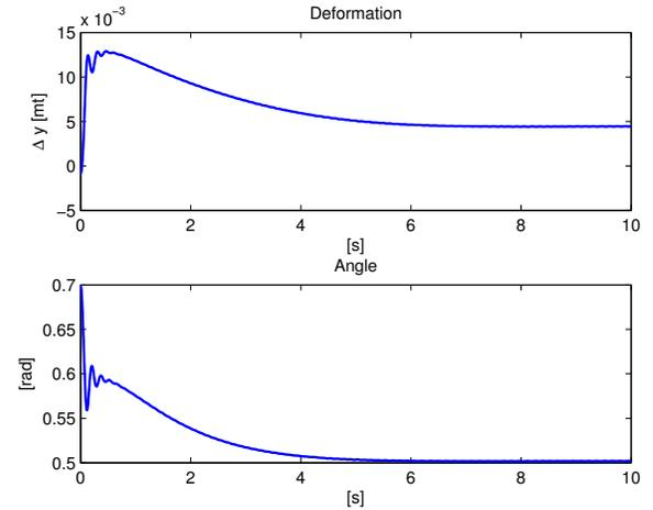
Fig. 6. Case 1: Soft finger-tip deformation (or penetration along its maximum radial deformation), top, and rolling angle convergence, bottom.
