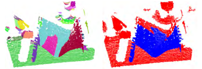
Fig. 13. Left: normal-based segmentation, displaying clusters in random color (with very small clusters deleted). Right: boundary-based segmentation, with a seed point in the center of the image. Please note that the red speckle in the middle is in the foreground, not part of the surface. Again, the same depth image as in Figure 1 is used. See text for details.
