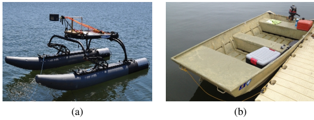
Fig. 6: (a) The autonomous USV14; (b) The human-controlled johnboat.
