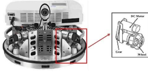
Fig. 1. Image of Robotino@ and its actuation subsystem.
