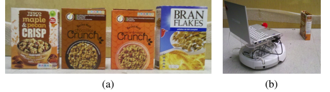
Fig. 1: (a) The boxes used for the search task. The similarity of the centre two leads to many identification errors. (b) The turtlebot examining a box during execution.
