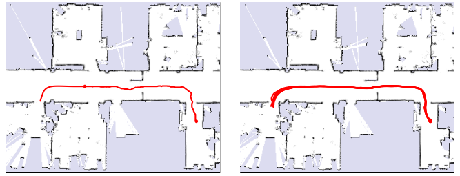
Fig. 3. Left: The trajectory that the robot has planned to travel to its target position. The trajectory from the current position of the robot to its intermediate goal is computed by our policy. The trajectory from the intermediate goal to the target position of the robot is computed by an A*-planner. Right: Trajectories driven by the robot using the policy learned by our approach. The robot successfully reached its goal position in 10 successive runs.
