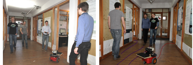
Fig. 1. Left: We teach a mobile robot an appropriate navigation behavior when interacting with humans via tele-operation. Right: Our approach learns a policy that allows the robot to autonomously navigate in a socially compliant way predicting the interaction behavior of nearby pedestrians.
