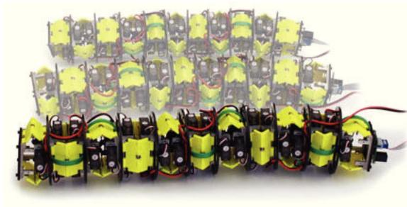
Fig. 12. Overlay of three stages in the rolling gait
