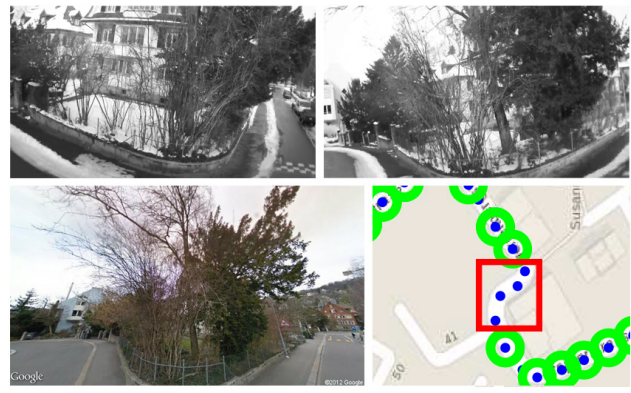
Fig. 10: Analysis in case of no detections. Top-left: urban MAV image; top-right: next view of the urban MAV; bottom-left: true positive pairing according to manual labeling; bottom-right: zoom on the global map, where the image was taken. Please note that these robot positions (top row) are difficult to be recognized even for humans. Moreover the over-season change of the vegetation makes it extremely difficult to cope with the pairing of them for image feature based techniques.
