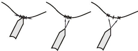
Fig. 3: (Left) Tight bidirectional path-following with vectors pointed at closely-spaced points on the path, (Center) vectors through the same points on the path guide the robot when the manipulator leaves the path, and (Right) more forgiving path following with more widely-spaced \delta^* vectors.
