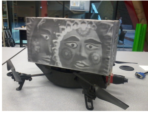
Fig. 2. The UAV used for visual servoing. At the pose shown, two faces of the cuboid are visible. Anyway, only the face with 'suns' should be used, since the other has a small visible area.
