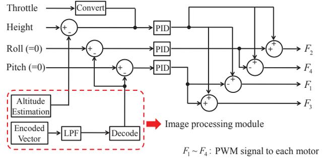
Fig. 8. Block diagram of attitude controller
