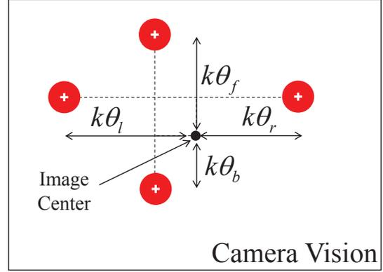
Fig. 6. Example of vision image when the quadrotor is tilted for both roll and pitch axes
