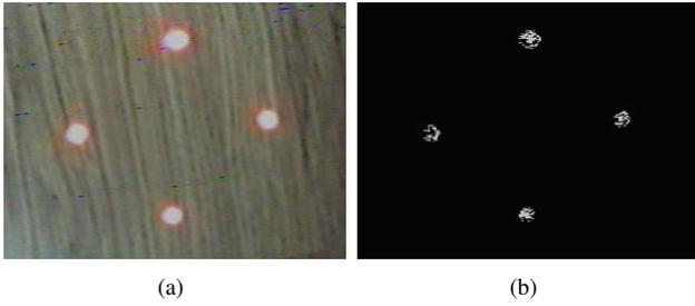
Fig. 4. Laser marker on the ground (a) original image from the vision sensor (b) converted image with HSV format
