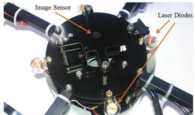
Fig. 3. Image sensor with laser diodes
