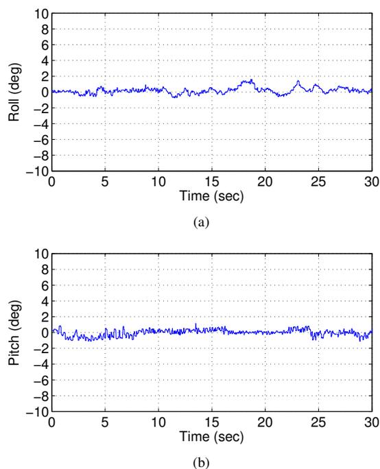
Fig. 10. Attitude data during stationary hovering (a) Roll angle (b) Pitch angle
