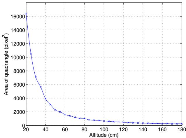
Fig. 12. Relationship between the altitude and the area of the quadrangle that is formed by the laser markers
