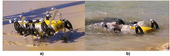
Fig. 1. a) Aqua robot walking on a beach with the Ninja legs. b) Aqua swimming in the sea water with the Ninja legs.
