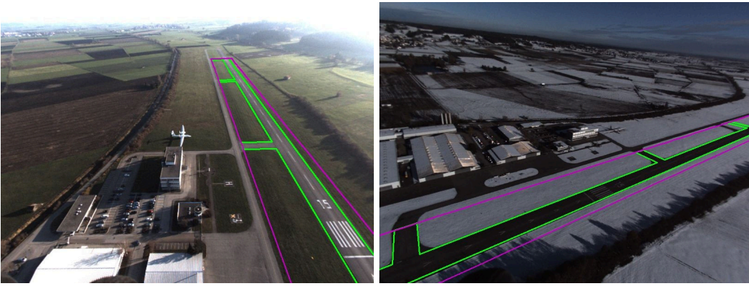
Fig. 7. Example images with detected runway recorded during flight experiments
