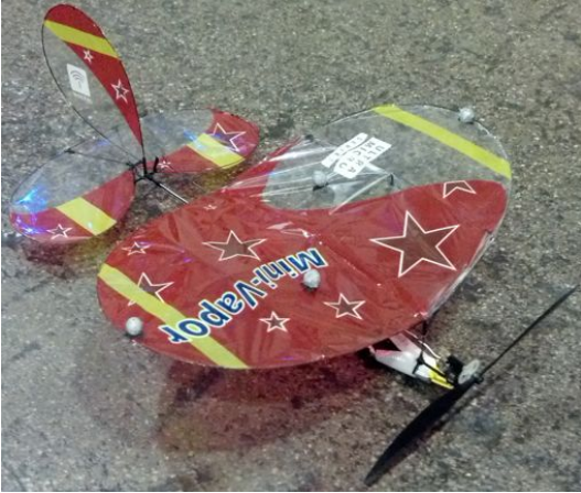
Fig. 11. An off-the-shelf MAV called MiniVapor. It has a rudder for yaw control, but no direct roll control mechanism.
