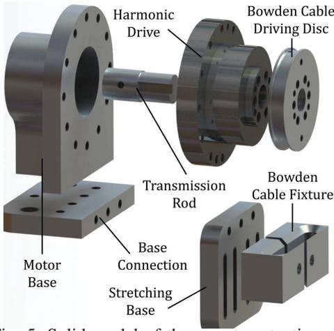
Fig. 5: Solid model of the remote actuation unit
