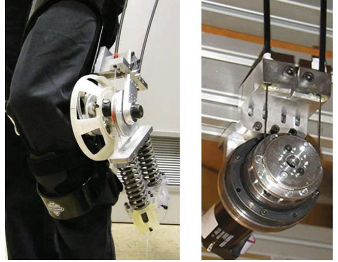
Fig. 7: ASSISTON-KNEE and its remote actuation unit
