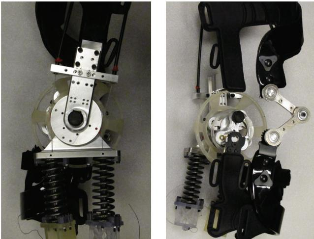
Fig. 6: Prototype of Bowden cable-driven series elastic ASSISTON-KNEE
