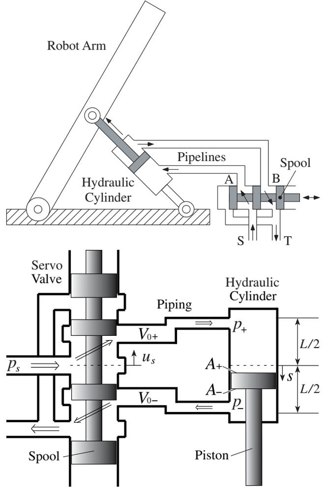
Fig. 1. The standard hydraulic arm (1-DOF case).
