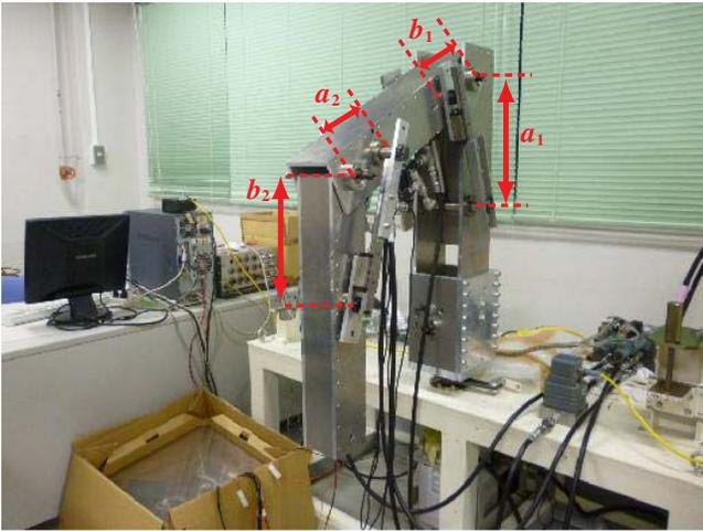
Fig. 2. The 2-DOF hydraulic robot with the design parameters  $(a, b)$
