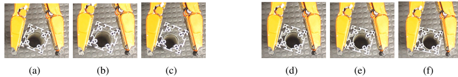
Fig. 13. Different grasp equilibria triggered by different levels of friction. The two sequences, left and right, show the evolution of two grasps starting from same initial conditions but yielding different final configurations thanks to two different levels of controlled friction. While on the left sequence high friction ensures stability for the initial grasping configuration, on the right a lower friction level let the grasped object slide in a different configuration.
