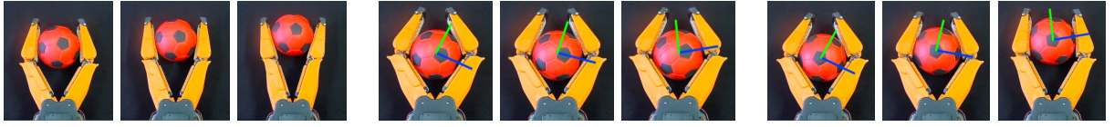
Fig. 4. In hand manipulation of a spherical object. The translation movement is obtained making the motors of the belts counter-rotate with the same angular speed (first three frames). By rotating the motors with the same intensity and direction, the ball is rotated (second three frames). The roto-translation movement is obtained actuating the motors with different in modulus angular speed (last three frames).
