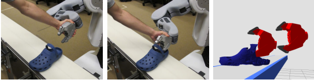
Fig. 2. From left to right, the user moves the end-effector to the pregrasp pose and then to the grasp pose. The pair of grasps is added to the database as they appear on the right.
