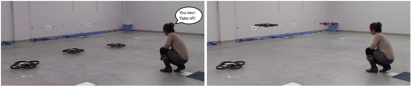
Fig. 1: An uninstrumented person selecting and commanding multiple robots out of a group by looking at them and saying the desired number of robots.
