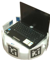
Fig. 1. iRobot Create with mounted Eee PC netbook for webcam use. Markers placed around the robot are used by neighboring robots to determine relative position and orientation
