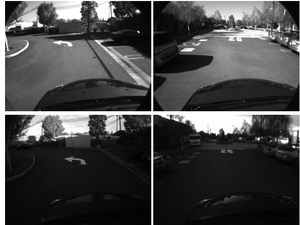
Fig. 4. Localization under change in lighting - We test and compare our system using two datasets with significant lighting change between them (top) dataset under good daylight conditions collected around 11am (bottom) dataset collected close to sundown.
