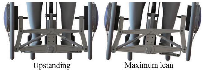
Fig. 8. Link mechanism for leaning
