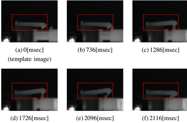
Fig. 8. Image of latch with impedance control under condition #1
