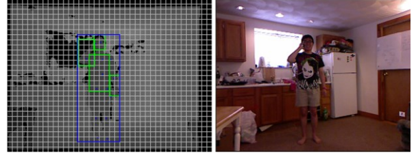
Fig. 2. We divide the whole depth image into blocks. And compute the histogram of oriented gradients for each block. The bounding boxes of body parts are computed according to joint positions, and add up the histograms of the blocks within the bounding box.
