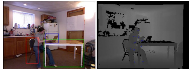
Fig. 1. The snapshot of working on computer of RGBD data from Kinect. We detect context information on RGB image, and extract skeleton features as well as Depth Histogram of Oriented Gradients (DHOG) features on depth image.
