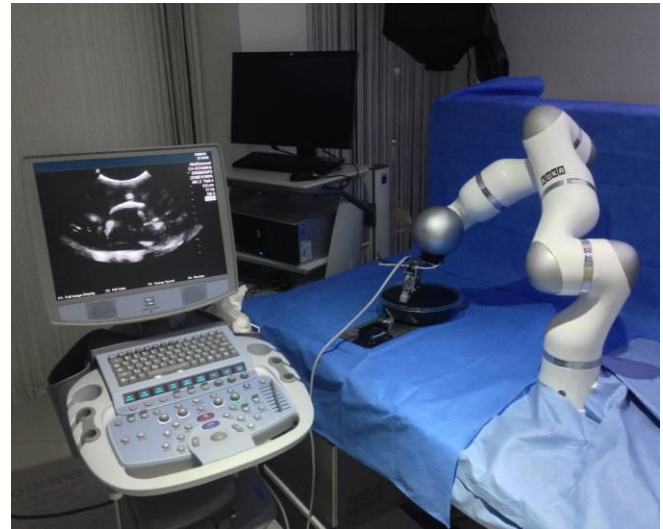
Fig. 1. On the left, the experimental setup used for the expert demonstration data collection is shown. The key components of the experimental setup are the medical ultrasound machine, an ultrasound phantom model and a handheld ultrasound transducer with force sensing and built-in 3D position markers. The respective optical-tracking camera is also shown on the background. On the right, the experimental setup used for the execution of the autonomous ultrasound routines learned by the proposed framework is shown. Here, the key component is the robotically controlled ultrasound probe which replaces the human operator.
