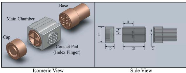
Fig. 2. The sections (*left*) and the internal structure (*right*) of the tactile display. All dimensions in the figure are in millimeters.
