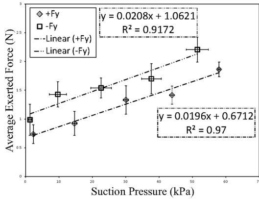
Fig. 7. Estimated tendency of exerted force in the y-axis (n=5).
