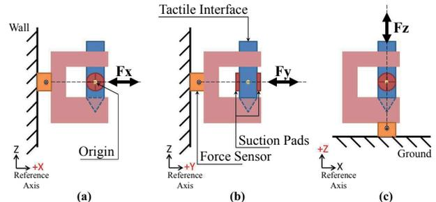
Fig. 4. Configurations of the experiment apparatus; (a)  $F_x$ , (b)  $F_y$ , and (c)  $F_z$ .
