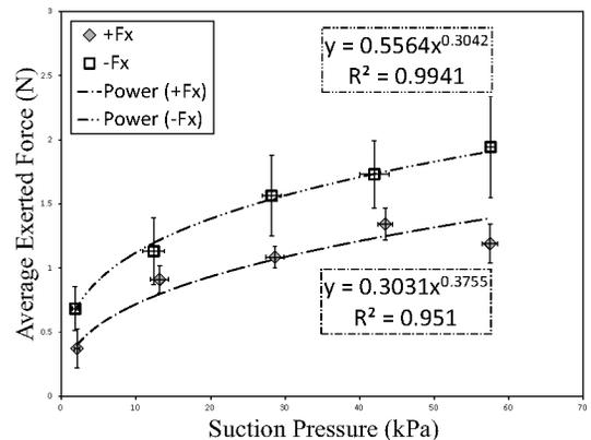
Fig. 6. Estimated tendency of exerted force in the x–axis (n=5).
