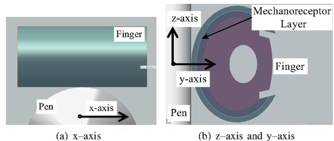
Fig. 9. Finite element model of the finger pad.
