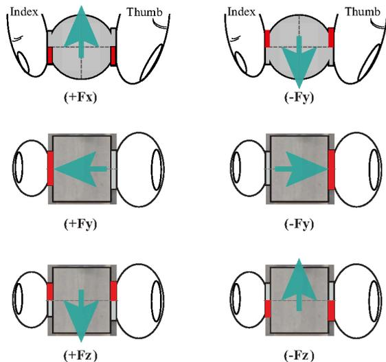
Fig. 5. Representation of force directions by suction pressure stimuli shown in red. These stimuli configurations are expected to evoke its respective representation of external force illustrated by the arrows.
