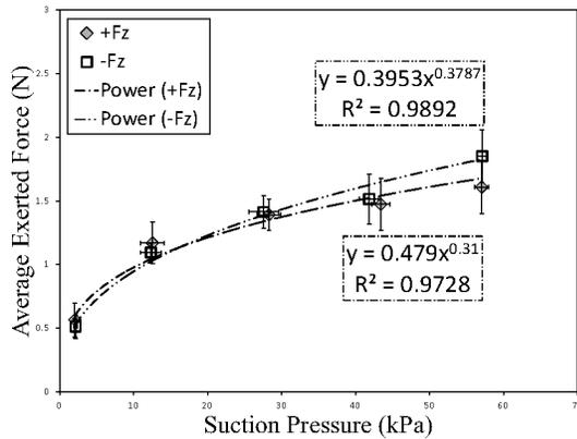
Fig. 8. Estimated tendency of exerted force in the z-axis (n=5).
