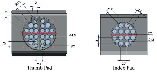
Fig. 3. The sizes and distribution of holes on the silicone rubber pads. All dimensions in the figure are in millimeters.
