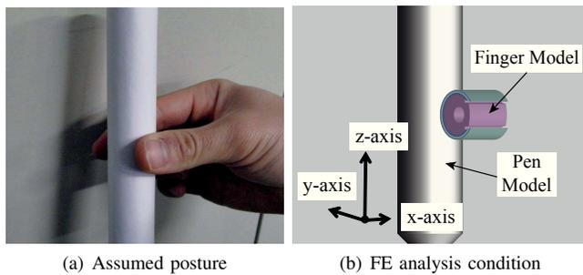
Fig. 10. Contact allocation between the finger and the pen.
