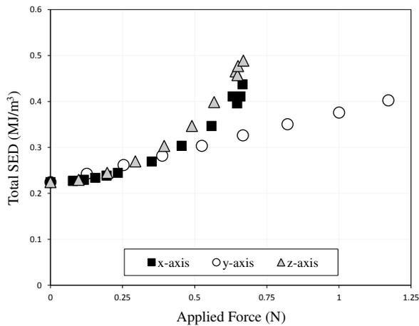
Fig. 12. Relationship between the total SED and the applied force.
