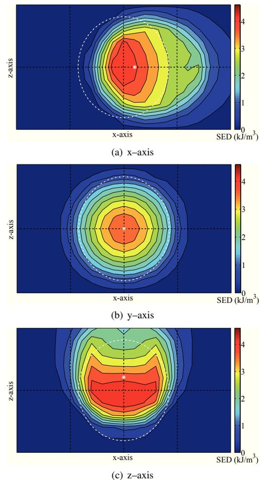
Fig. 11. SED distribution when the external force of 0.65 N is applied to the three directions
